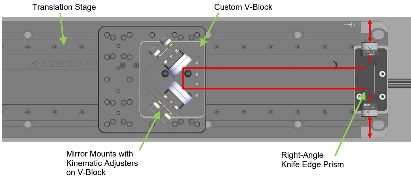
**Figure 2 Schematic of an Optical Delay Line Kit**
