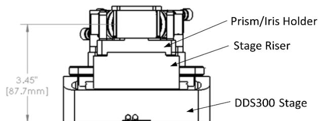
**Figure 4** Mounting the Stage Riser and Knife-Edge Prism
